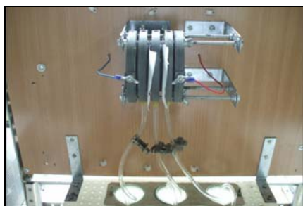
Fig. 1. The experimental electrodialysis cell with three compartments
