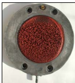
Fig. 4. The metallic copper layer deposited onto the cathode.
