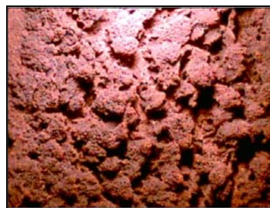
Fig. 5. Microscopic image 60 X of copper deposited onto the Pb electrode.
