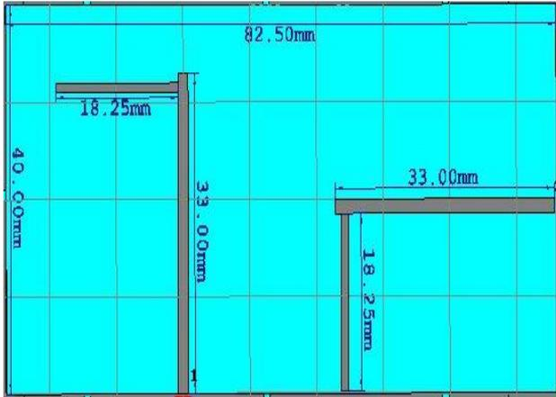
Fig. 1. The size and geometry of the antenna that is proposed in the study
