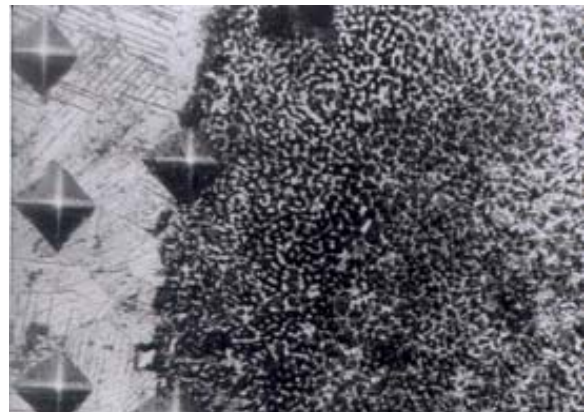
Fig. 7. Penetrator imprints for 21MoMnCr12.
