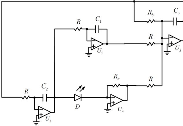
Fig. 1. Schematic of the circuit in which the light-emitting diode is denoted as  $D$
