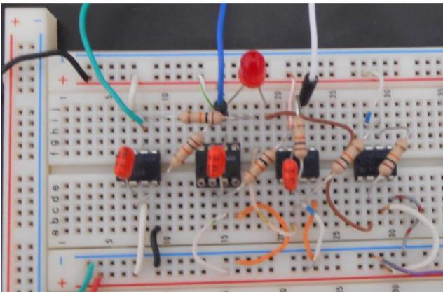
Fig. 9. Implemented circuit in breadboard in which the red light-emitting diode can be used to display the chaotic flicker of the light
