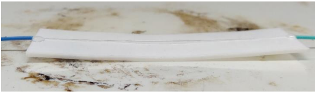
Fig. 9. The bending of PTFE material on one-sided packaging (color online)
