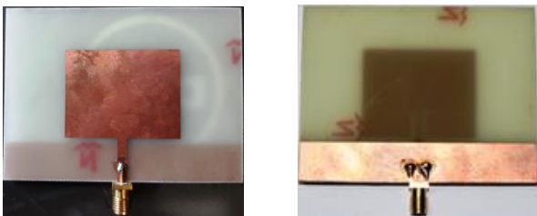
Fig. 4. Prototype of the designed antenna (color online)
