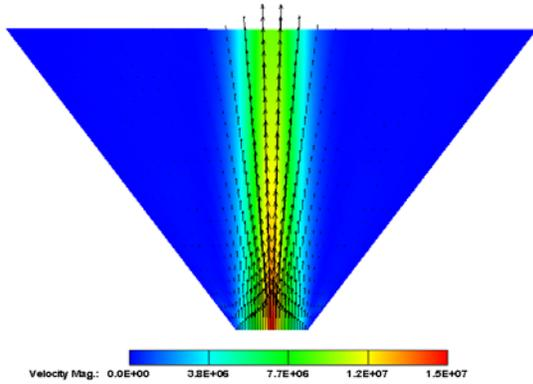
Fig. 5. The fluid velocity along the diffuser, with the vectors representation; velocity is expressed in  $\mu\text{m/s}$ .
