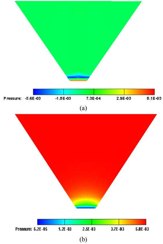
Fig. 6. The pressure distribution in MPa: (a) The diffuser case; (b) The nozzle case.
