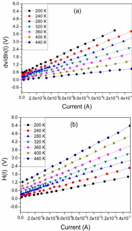
Fig. 4. (a) Plots of  $dV/d\ln(I)$  versus  $I$ , and (b)  $H(I)$  versus  $I$  for Pt/Ti/n-InP Schottky diode.
