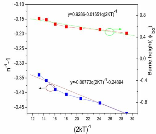
Fig. 6. The zero-bias apparent barrier height and ideality factor versus  $1/2kT$  curves of the Pt/Ti/n-InP Schottky diode according to Gaussian distribution.
