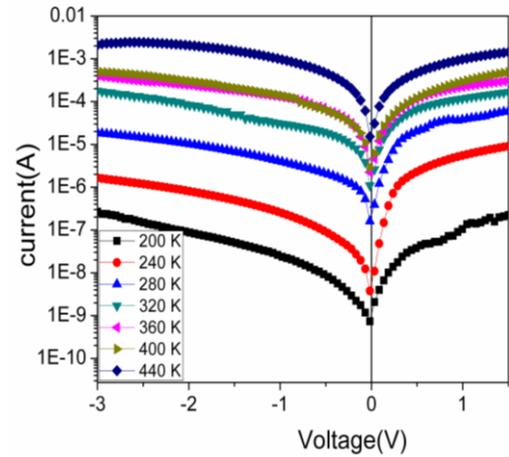
Fig. 1. Experimental reverse and forward-bias current-voltage (I-V) characteristics of Pt/Ti/n-InP Schottky diode in the temperature range of 200-440 K.
