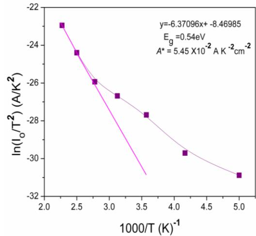
Fig. 3. Richardson plot for  $\ln(I_o/T^2)$  versus  $1000/T$  for Pt/Ti/n-InP Schottky diode.
