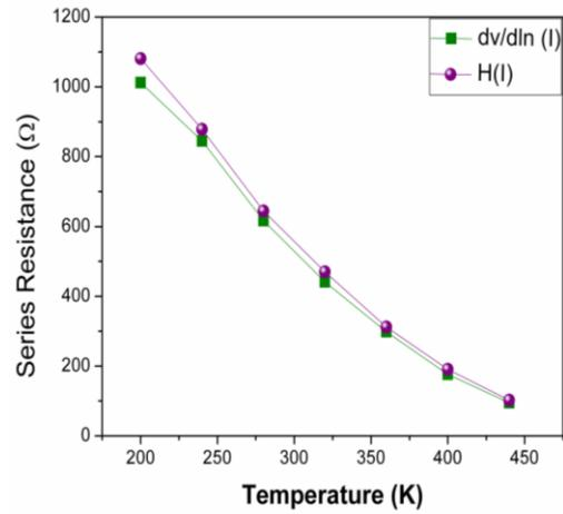
Fig. 5. Temperature dependence of the series resistances obtained from Cheung's method for Pt/Ti/n-InP Schottky diode.
