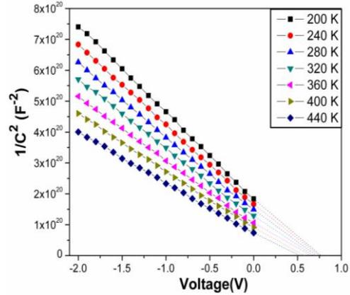
Fig. 8. The reverse bias C<sup>-2</sup>-V characteristics of the Pt/Ti/n-InP Schottky diode at different temperatures in the range 200-440 K.
