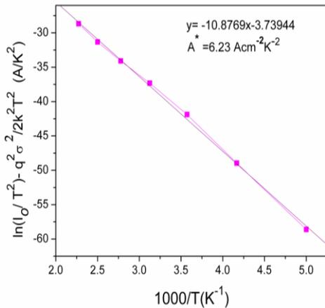
Fig. 7. Modified Richardson plot for the Pt/Ti/n-InP Schottky diode according to Gaussian distribution of the barrier heights.
