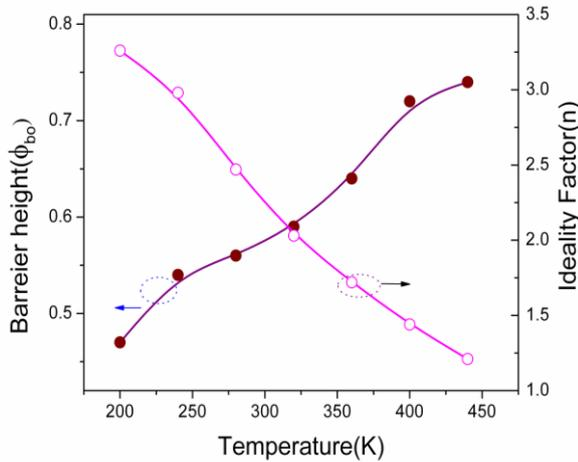
Fig. 2. Temperature dependence of the ideality factor and barrier height for Pt/Ti/n-InP Schottky diode.
