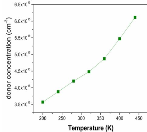
Fig. 9. Temperature dependence of the carrier concentration from experimental reverse bias C<sup>-2</sup>-V characteristics for the Pt/Ti/n-InP Schottky diode.
