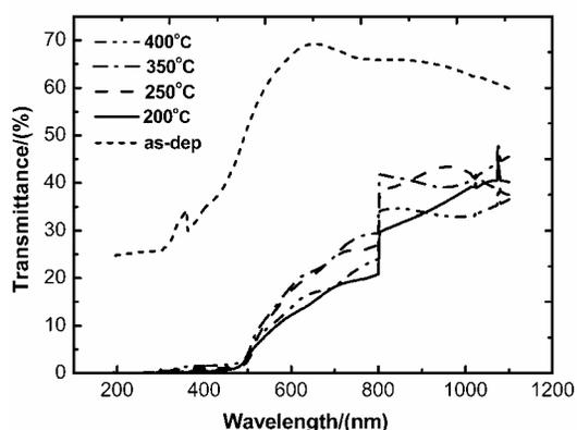
Fig. 4. Transmittance spectra curves of  $\text{CuInSe}_2$  films prepared with various annealing temperatures.
