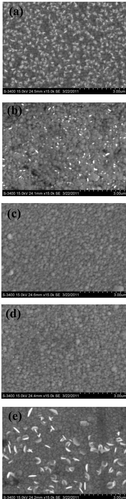
Fig. 2. SEM images of cross sections in CuInSe<sub>2</sub> films prepared at various annealing temperatures: (a) as-deposited; (b) 200 °C; (c) 250 °C; (d) 350 °C; (e) 400 °C
