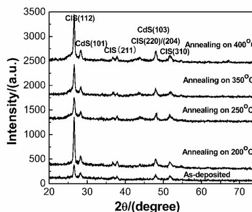
Fig. 1. XRD patterns of CuInSe<sub>2</sub> films prepared at various annealing temperatures.
