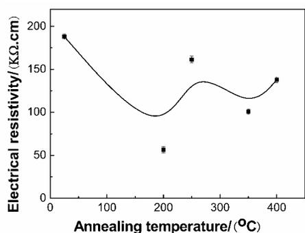
Fig. 3. The resistivity curves of  $\text{CuInSe}_2$  films as a function of the annealing temperatures.
