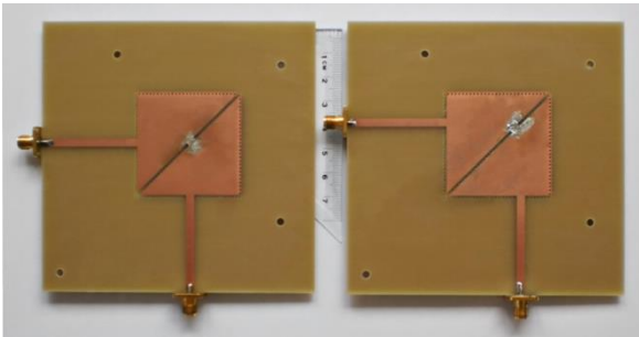
Fig. 9. Photograph of the two filters fabricated on FR4 substrate Filter 1 (left) and Filter 2 (right)
