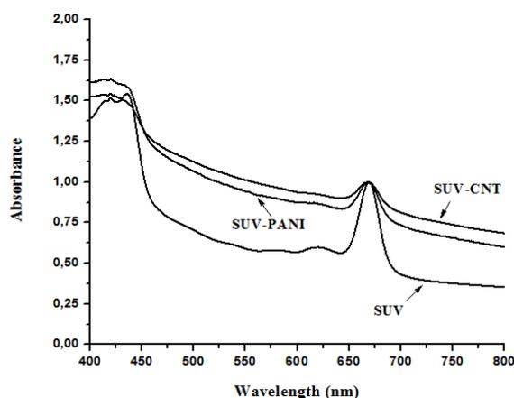
Fig. 2. The Vis absorption spectra of Chla in SUV liposomes and in bioconposites (SUV-CNT and SUV-PANI)
