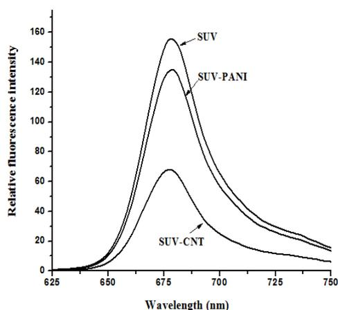
Fig. 3. Fluorescence emission spectra of Chla in DPPC (0.5 mM) liposomes and in biocomposites: Chla-DPPC (0.5 mM) liposomes/SWCNTs & Chla-DPPC (0.5 mM) liposomes/PANI (excitation wavelength: 430 nm)
