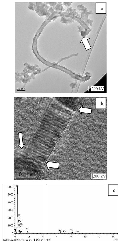
Fig. 4. TEM image of annealed graphite at  $1600^{\circ}\text{C}$  for 6 h. a), b) CNTs, c) EDX of structure at the end of the CNTs.
