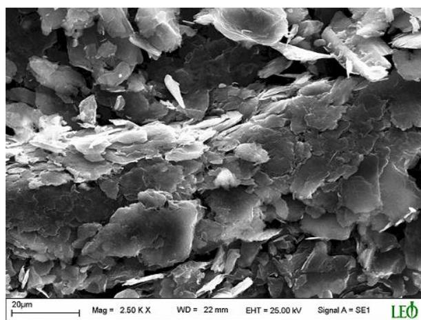
Fig. 2. SEM image of powders wet milled and then annealed at 1600 °C for 6 h.
