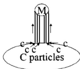
Fig. 5. Schematic illustrations of the growth mechanism proposed for solid-state formation [7].
