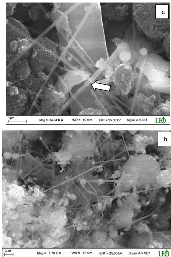
Fig. 3. SEM image of annealed graphite at  $1600^{\circ}\text{C}$  for 6 h. a) Bamboo type CNTs, b) metal based various structures at the end of the CNTs.
