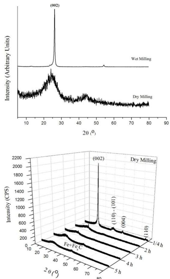
Fig. 1. XRD patterns of a) dry and wet milled powders for 5 h, b) dry milling for 1/4, 2, 3, 4, 5 h.
