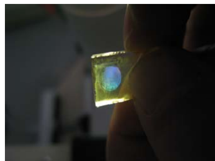
Fig. 14. Demonstration of light diffraction by the grating resulted from recording laser radiation ( Ar ) after developing.
