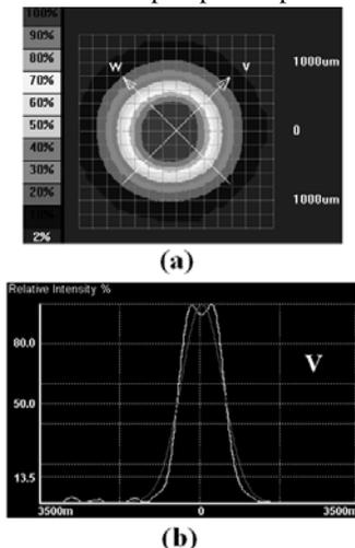
Fig. 2. Measured intensity distribution of pump modes with normal coiling. (a) 2D intensity profile; (b) radial intensity variation along the V axis. The reference line is Gaussian fit profile.
