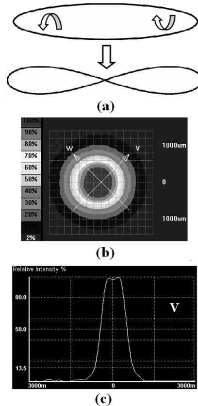
Fig. 3. (a) Schematic diagram of twisting the normal fiber spool. Measured intensity distribution of pump modes with mode scrambling: (b) 2D intensity profile; (c) radial intensity variation along the V axis.
