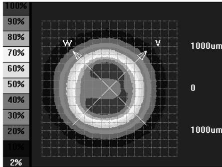
Fig. 4. Measured 2D intensity profile of pump modes with the deterioration of pump coupling efficiency.
