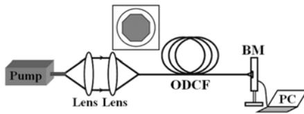
Fig. 1 Experimental setup. ODCF: Octagonal double-clad fiber. BM: BeamMaster. PC: Personal computer. The inset shows the cross section of ODCF.
