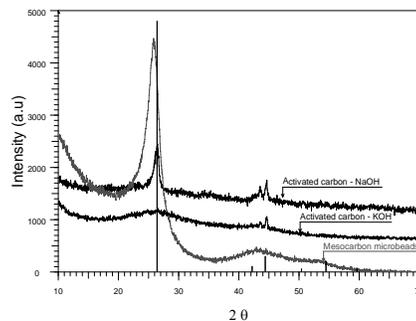
Fig. 3. XRD pattern of: MCMB, activated MCMB with NaOH, activated MCMB with KOH
