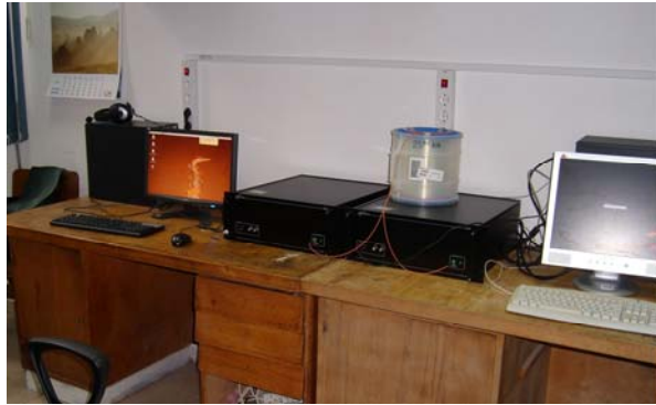
Fig. 2. Communication line setup used in the QUANTGRID D11-044 project (Inst. For Laser and Plasma Phys. – Bucharest), with its two dedicated computers (Bob – receiver and Alice – sender). The quantum channel (23.845 km) optical fiber spool is on top of the Bob station. The classical channel linking the computers is local LAN Ethernet.
