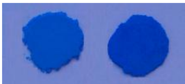
Fig. 6. Image of Zn_{1-x}Co_xAl_2O_4 pigment where x = 0.05 (left), x = 0.1 (right) annealed at 1000^\circ C .
