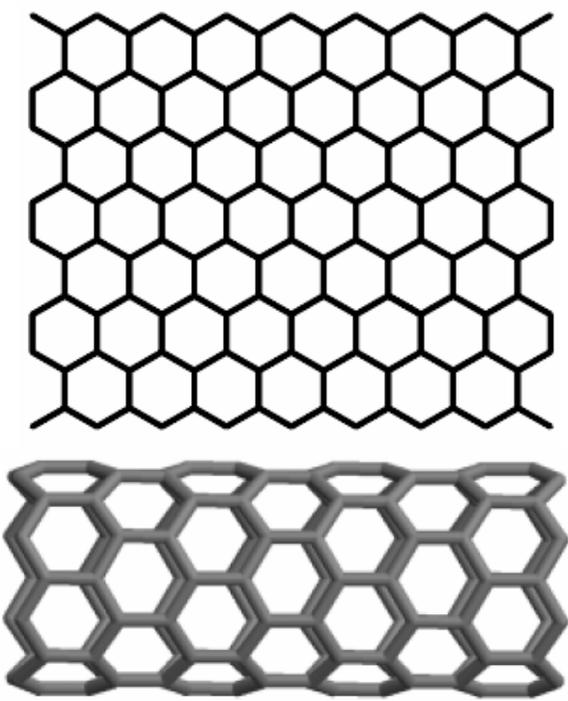
Fig. 2. 2-dimensional lattice of nanotube  $TUZC_6 [8,4]$ .
