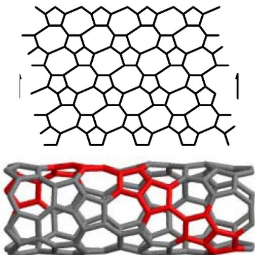
Fig. 4. 2-dimensional lattice of nanotube  $SC_5C_7 [8,4]$ .
