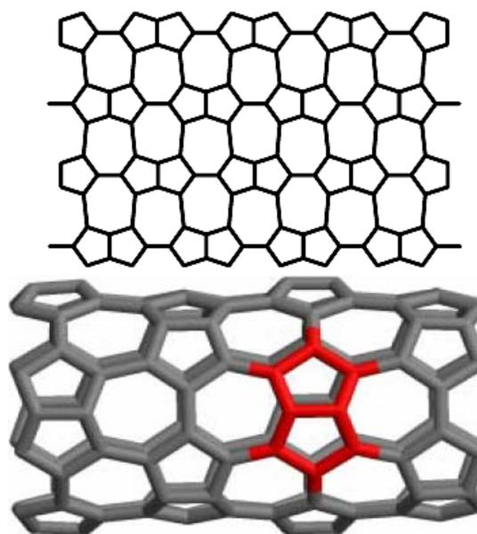
Fig. 3. 2-dimensional lattice of nanotube  $HC_5C_7 [8,4]$ .
