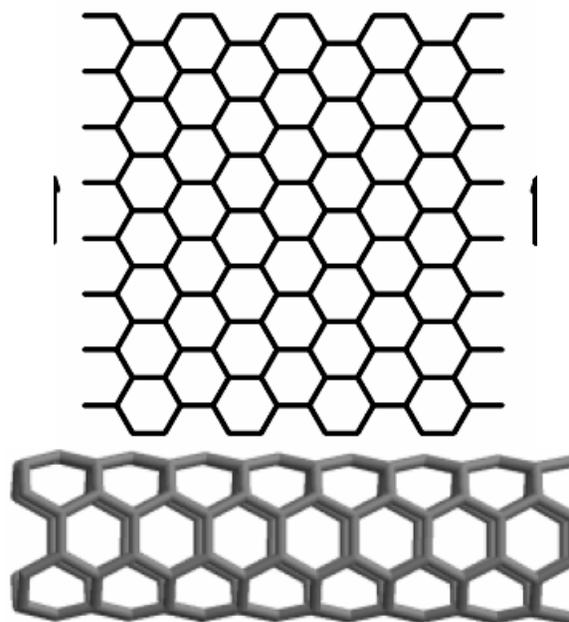
Fig. 1. 2-dimensional lattice of nanotube TUAC<sub>6</sub> [4,8].
