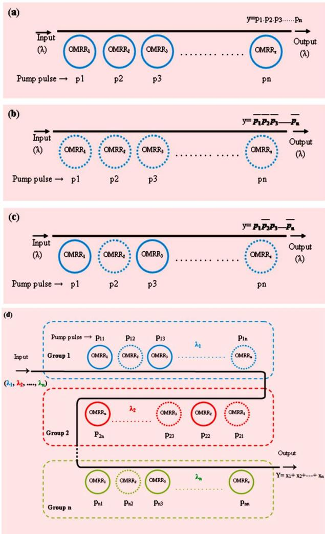
Fig. 3. Logic circuit of (a) OMRRs working in off/on mode with single working wavelength, (b) OMRRs working in on/off mode with single working wavelength, (c) OMRRs working in the on/off or off/on mode with single working wavelength and, (d) the proposed reconfigurable logic circuit. The solid line ring resonator indicates OMRR works in the off/on mode, the dot line ring resonator indicates OMRR works in the on/off mode, OMRRs with the same color work at the same working wavelength
