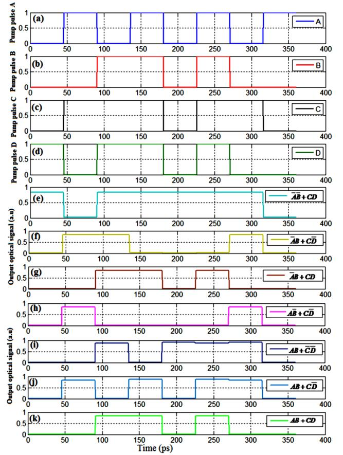
Fig. 6. Simulation results of reconfigurable logic circuit with four-operand; ((a)–(d)) represent the optical pump pulses applied to OMRRs, and ((e)–(k)) represent different logic operation results
