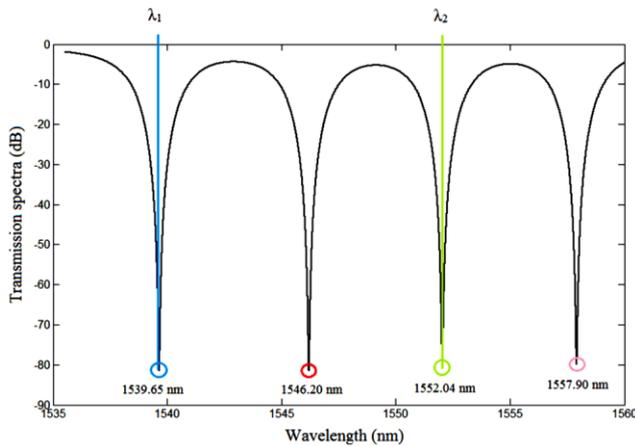
Fig. 4. The spectral response of the device with no pump pulse applied to OMRRs
