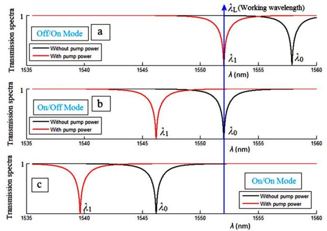
Fig. 2. The transmission spectra of a switch for light with the wavelength of  $\lambda_L$  (a) in off/on mode, (b) in on/off mode, (c) in on/on mode
