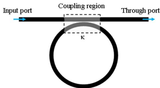
Fig. 1. Single waveguide coupled micro-ring resonator
