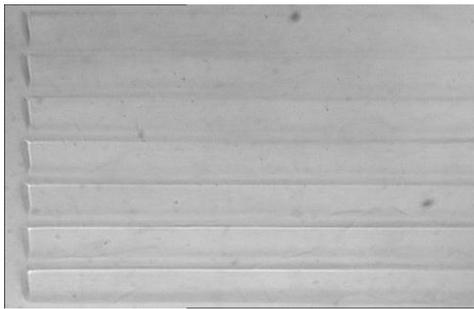
(a) Optical microscopy image ( $\times 400$ ) of  $64\mu\text{m}$  period
