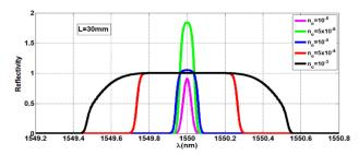
Fig. 6. Reflectivity spectrum for Blackman apodization profile at L= 30 mm
