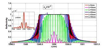
Fig. 9. Reflectivity of the sigmoid apodization profile at  $n_o = 10^{-3}$
