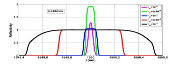
Fig. 4. Reflectivity of raised cosine apodization profile at L= 30 mm
