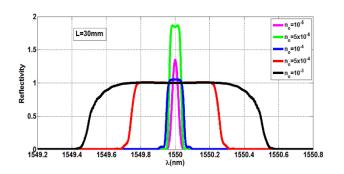
Fig. 8. Reflectivity spectrum for the Bartlett apodization profile at L= 30 mm
