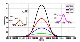
Fig. 7. Reflectivity spectrum for the Bartlett apodization profile at  $n_o = 10^{-5}$
