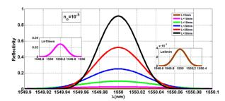
Fig. 5. Reflectivity spectrum for Blackman apodization profile at  $n_o = 10^{-5}$
