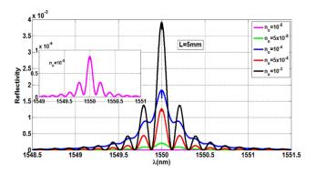
Fig. 10. Reflectivity of the sigmoid apodization profile at L = 5 mm
