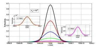
Fig. 11. Reflectivity spectrum for the Nuttall apodization profile at  $n_o = 10^{-5}$
