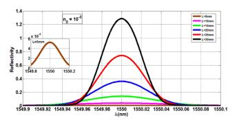
Fig. 3. Reflectivity spectrum for a raised cosine apodization profile at no=10-5
