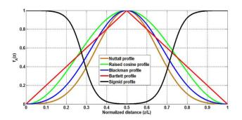
Fig. 2. FBG Apodization profiles for DFB-F
