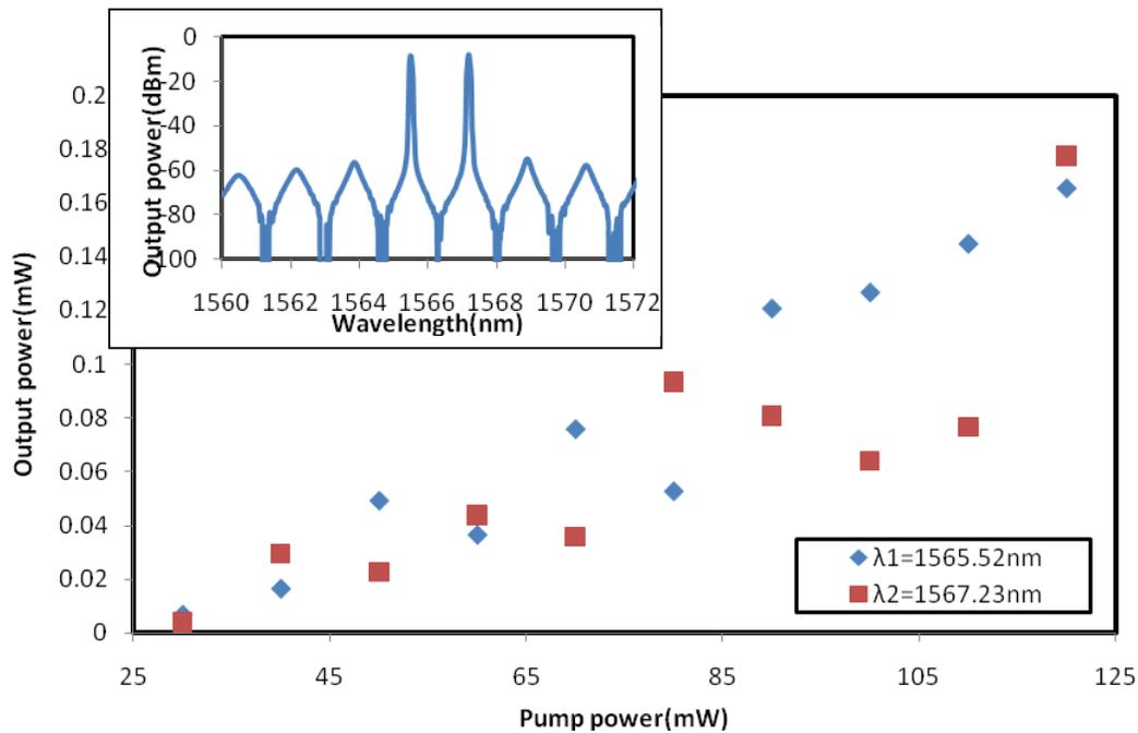
Fig. 2. The output laser power against 1480 nm pump power for both lasing lines. Inset shows the output spectrum of the dual-wavelength laser at 120 mW pump power.
