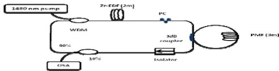
Fig. 1. Schematic diagram of the setup for dual wavelength ring laser utilized EDZF.
