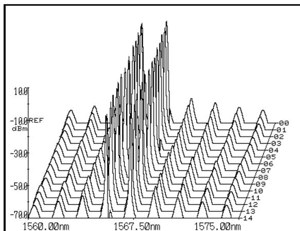
Fig. 3. Spectral evolutions of the proposed dual-wavelength EDZF laser against time. (The laser spectrum was scanned at every 5 minutes).
