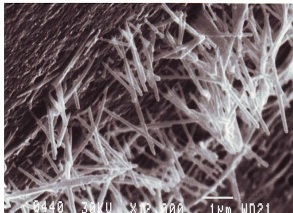
Fig. 2. SEM micrograph of 100 nm silver iodide nanowires.
