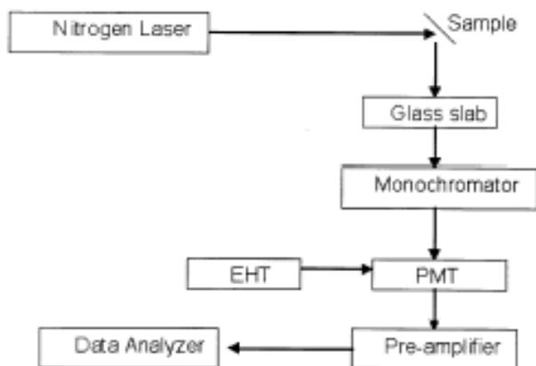
Fig. 1. Photoluminescence setup.
