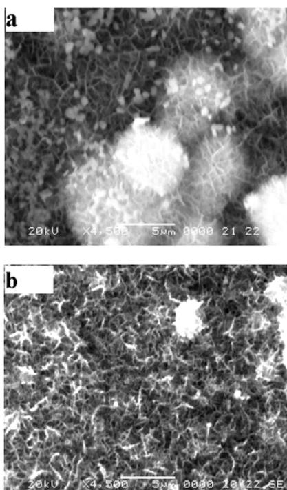
Fig. 1. SEM micrograph of CdS nanorod/nanowire after chemical etching (a) for 5 second (b) for 15 second.
