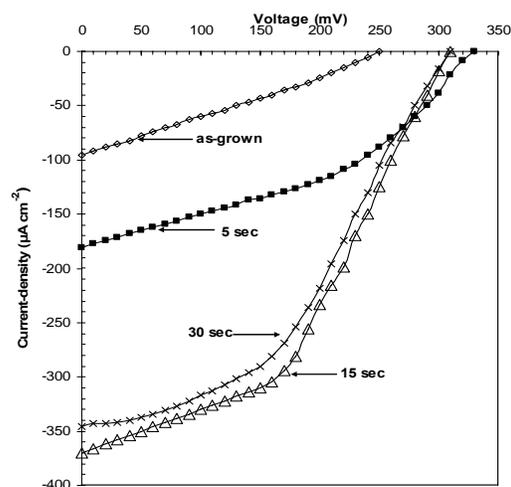
Fig. 5. Photovoltaic output characteristics for n-CdS/IM (NaOH-Na<sub>2</sub>S-S)/C PEC cells of (a) as-grown (b) after 5 sec etching (c) after 15 sec etching (d) after 30 sec etching.
