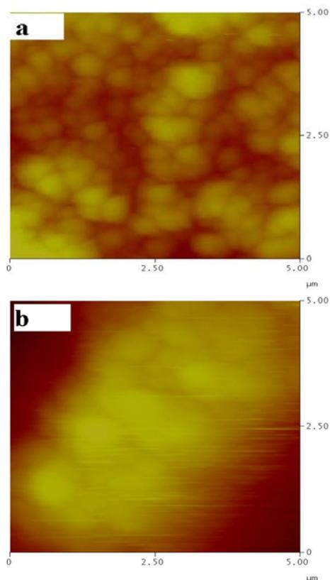
Fig. 2. AFM image of CdS nanoparticles (a) as-grown and (b) annealed at 473K.
