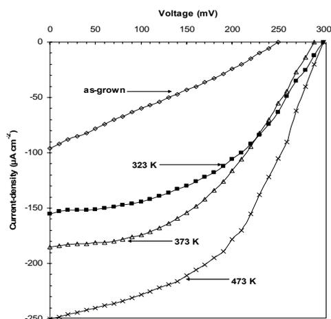
Fig. 6. Shows photovoltaic output characteristics of the as-grown and annealed (373, 423 and 473K for 1 hrs) CdS film photoelectrodes.
