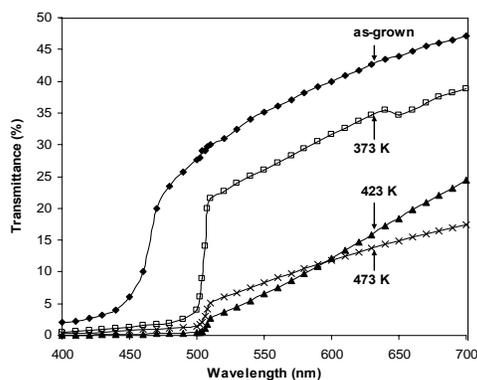
Fig. 3. Optical transmission spectra of as-grown and annealed (at 373, 423 and 473 K for 1 hrs) CdS thin films.
