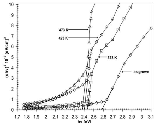
Fig. 4. Variation of  $(ahv)^2$  with energy of as-grown and annealed (at 373, 423 and 473 K for 1 hrs) CdS thin films.
