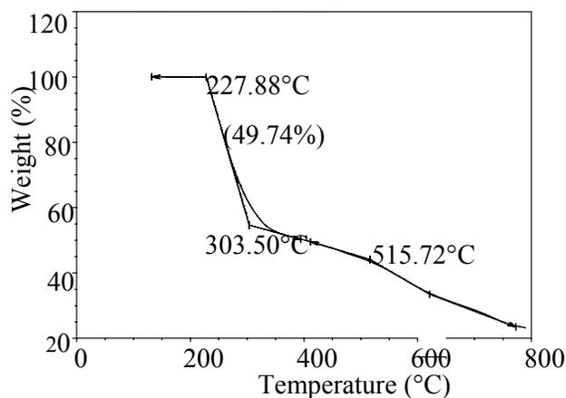
Fig.6 . TGA thermogram of Glycine doped ZTC Crystal
