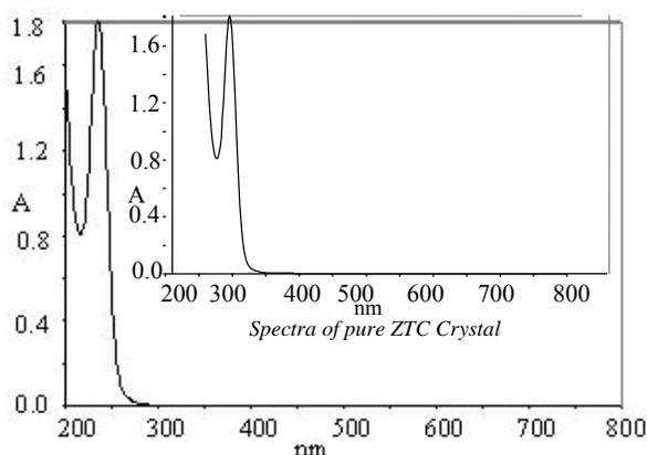
Fig. 5. UV-Vis absorbance spectra of Glycine doped ZTC Crystal.
