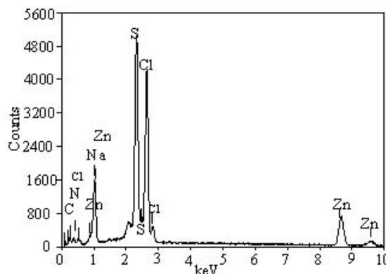
Fig. 4 EDAX spectrum of Glycine doped ZTC Crystal.
