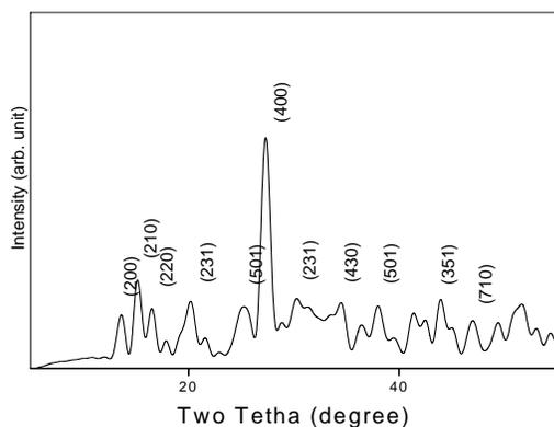
Fig. 2. Powder XRD pattern (the numbers assigned to various peaks are values of hkl indexes)
