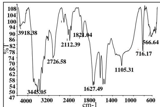
Fig. 3(b). FTIR spectrum of Glycine doped ZTC Crystal.
