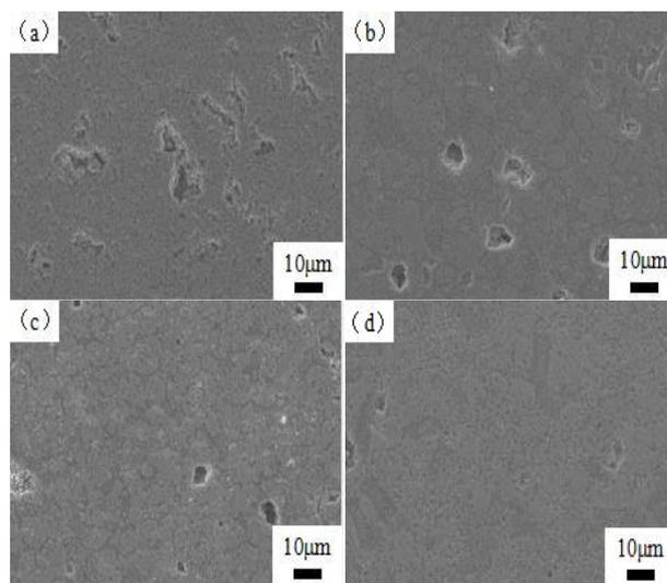
Fig. 3. SEM images of samples crystallized at (a) 1200 °C, (b) 1210 °C, (c) 1220 °C, (d) 1230 °C
