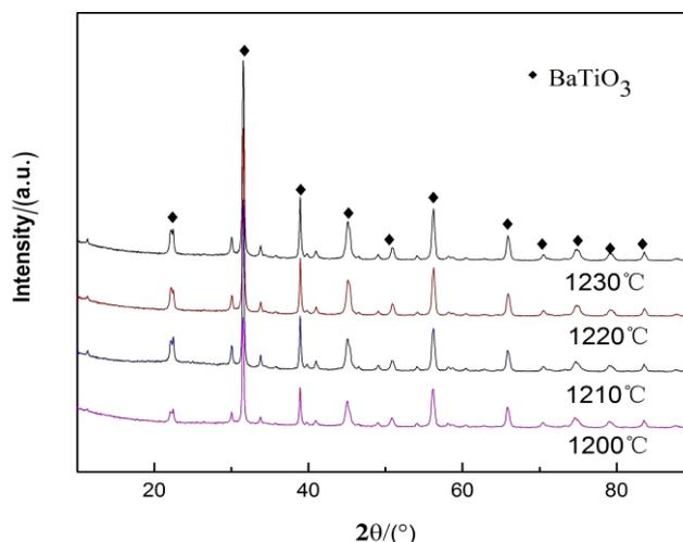
Fig. 2. XRD patterns of samples crystallized at different Temperatures
