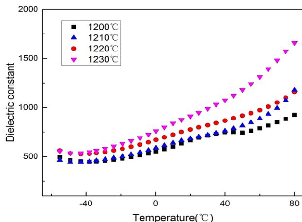
Fig. 5. Dielectric constant as a function of testing temperature for the samples crystallized at different temperatures (measured at 1 kHz)
