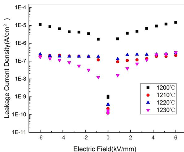
Fig. 6. Leakage current curves of the glass-ceramics samples crystallized at different temperatures
