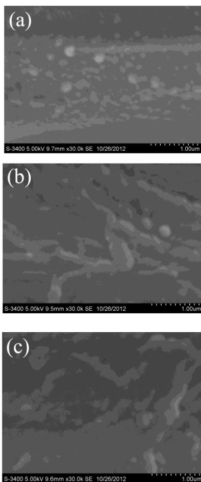
Fig. 3. High multiples ( $\times 30$  k) of SEM images of Al films deposited on various substrates: (a) Polyester; (b) Cotton and (c) Aramid.
