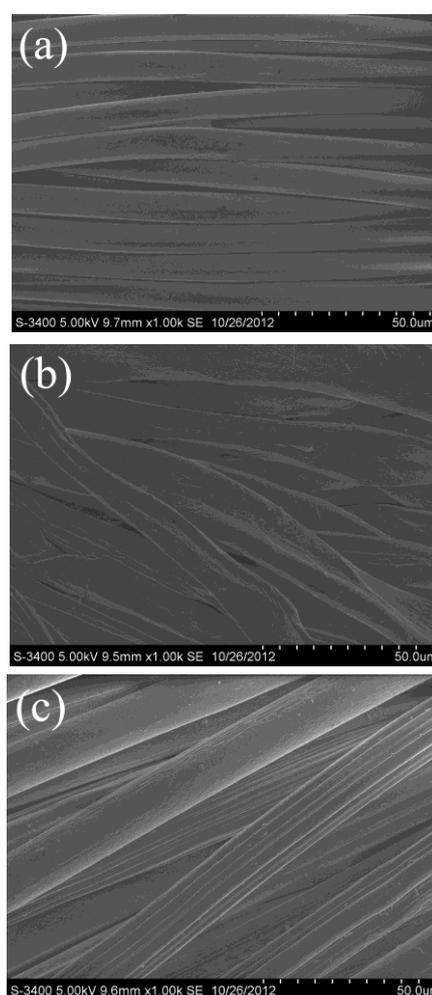
Fig. 2. Low multiples ( $\times 1k$ ) of SEM images of Al films deposited on various substrates: (a) Polyester, (b) Cotton and (c) Aramid.
