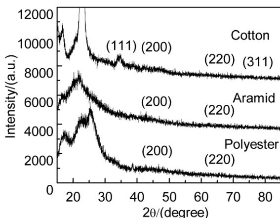
Fig. 1. XRD patterns of Al films prepared on various substrates.
