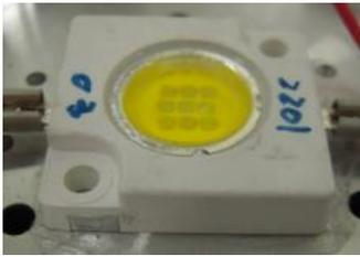
Fig. 1. The experimental WLED having CCT of 8500 K
