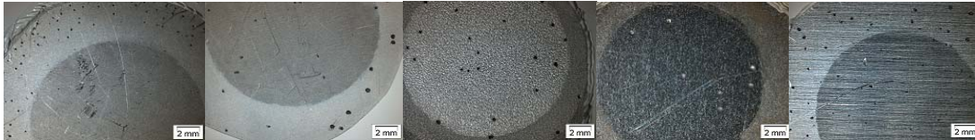
Fig. 8. The appearance of the samples from the potentiostatic measurements, I_h by 800 mV(SHE).
