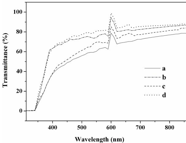
Fig. 4. Transmittance spectra of the ZnO: Al films (a) preannealed at 400 °C and annealed at 600 °C, (b) direct annealed at 700 °C, (c) preannealed at 400 °C and annealed at 700 °C, (d) annealed at 700 °C.
