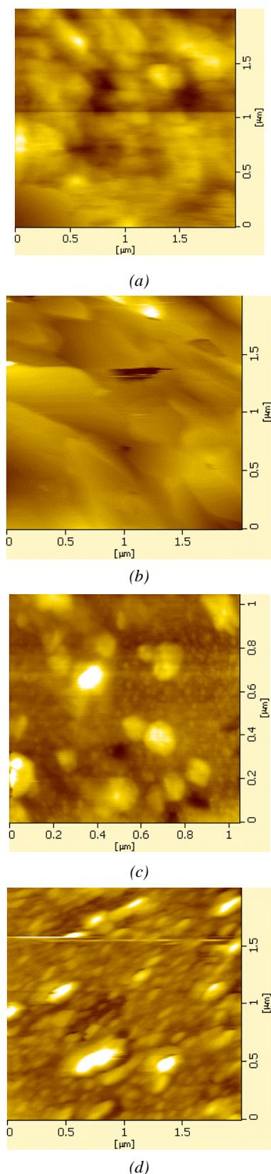
Fig. 3. AFM micrographs of the five layer ZnO: Al films (a) preannealed at 400 °C and annealed at 600 °C, (b) direct annealed at 700 °C, (c) preannealed at 400 °C and annealed at 700 °C, (d) annealed at 700 °C.
