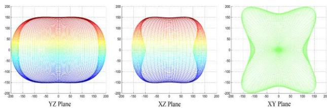
Fig. 3. The projection of Young's modulus (GGA results) in different planes for Pnma  $YFeO_3$ .
