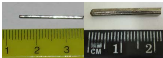
Fig. 3. The rods prepared by mould casting.
