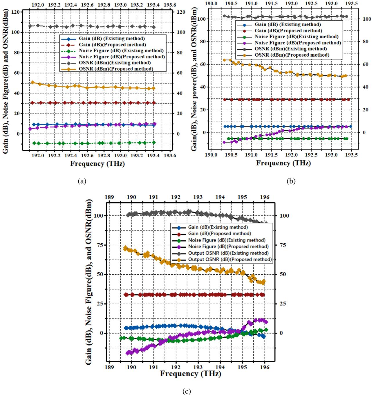
Fig. 5. Existing and Proposed method comparison of Gain, Noise Figure and OSNR for (a) 16- channel, (b) 32-channel, and (c) 64-channel configurations (color online)
