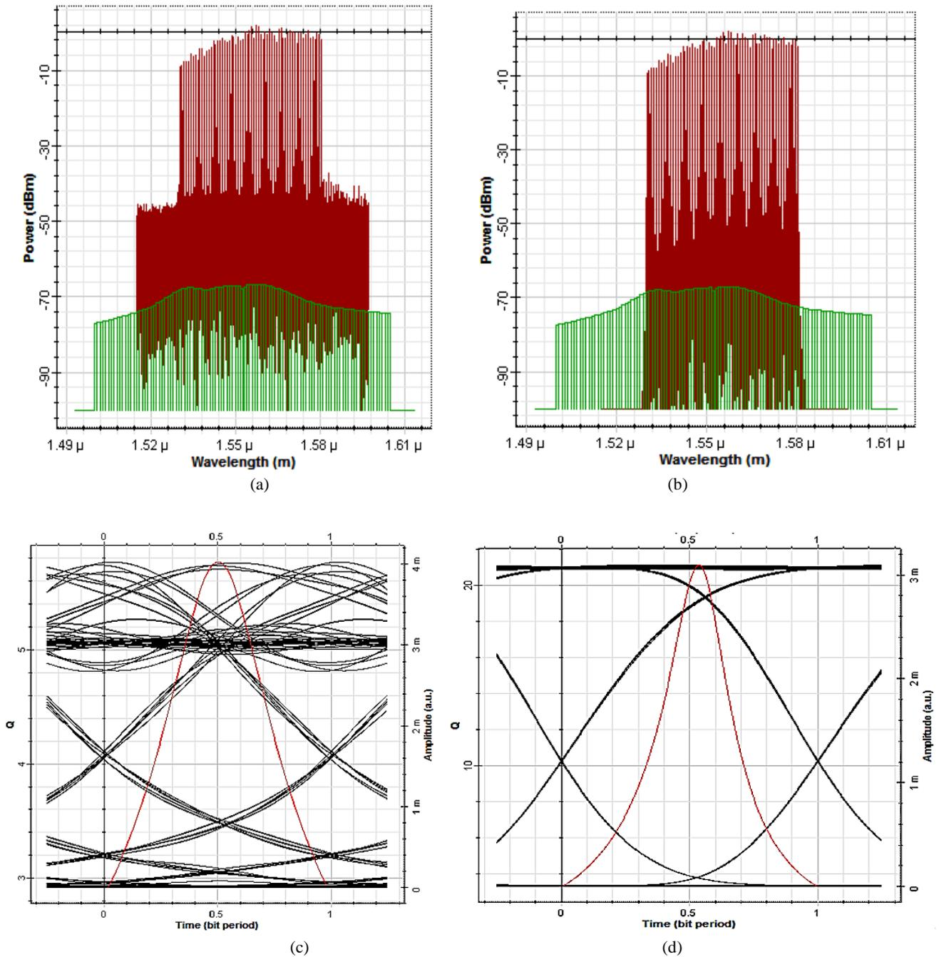
Fig. 4. The spectrum analyzer output (a) Existing and (b) the proposed method. BER analyzer output (c) Existing and (d) proposed method (color online)
