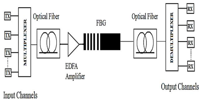
Fig. 1. Wavelength division multiplexing system with FBG
