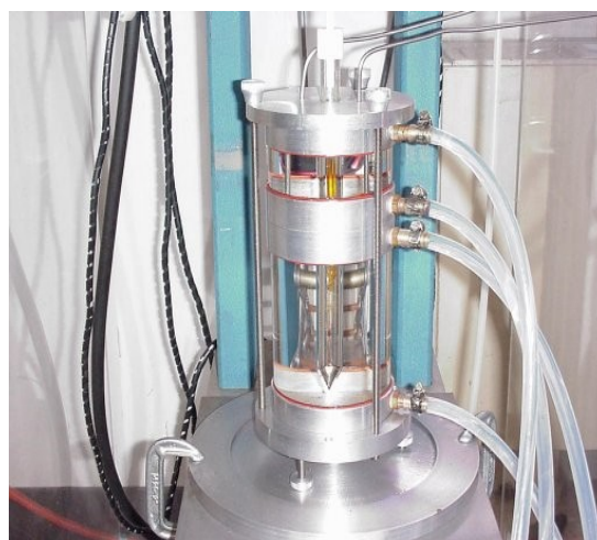
Fig. 2. A photograph of modified Bridgman Stockbarger (BS) set-up.
