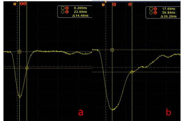
Fig. 8. The decay time spectrum of 0.5mol% Tm<sup>3+</sup> doped BSO crystal, a) Fast component; b) Slow component (color online)
