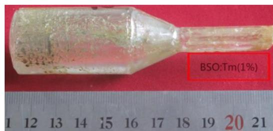
Fig. 1. The  $(\text{Bi}_{0.99}\text{Tm}_{0.01})_4\text{Si}_3\text{O}_{12}$  crystal grown by the modified vertical Bridgman method
