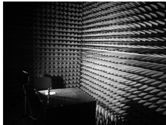
Fig. 1. The anechoic chamber.
