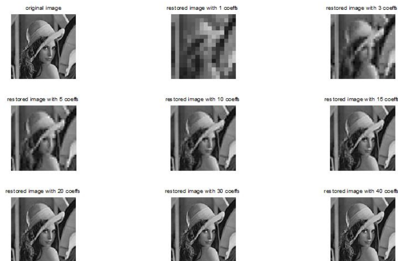
Fig. 6. Lena image restored using various numbers of coefficients.
