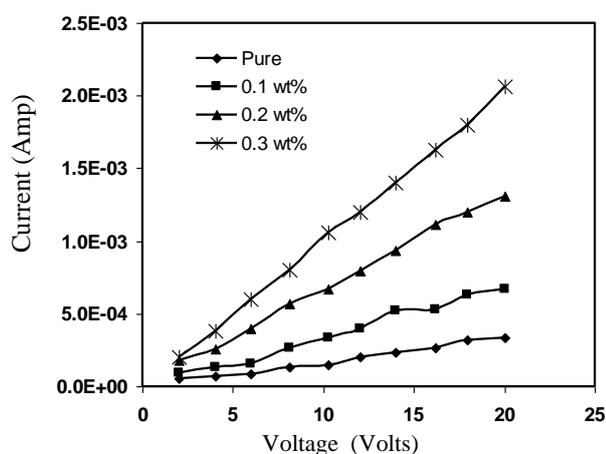
Fig. 4. The I-V curves for POT and POT-MWCNTs with different MWCNTs weight ratios
