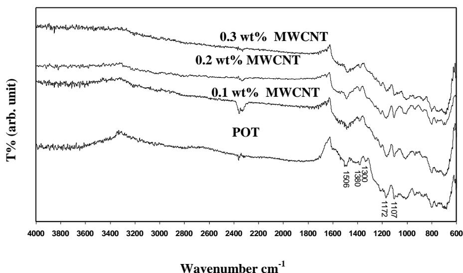
Fig. 3. FTIR spectra of POT and POT-MWCNTs with different MWCNTs weight ratios
