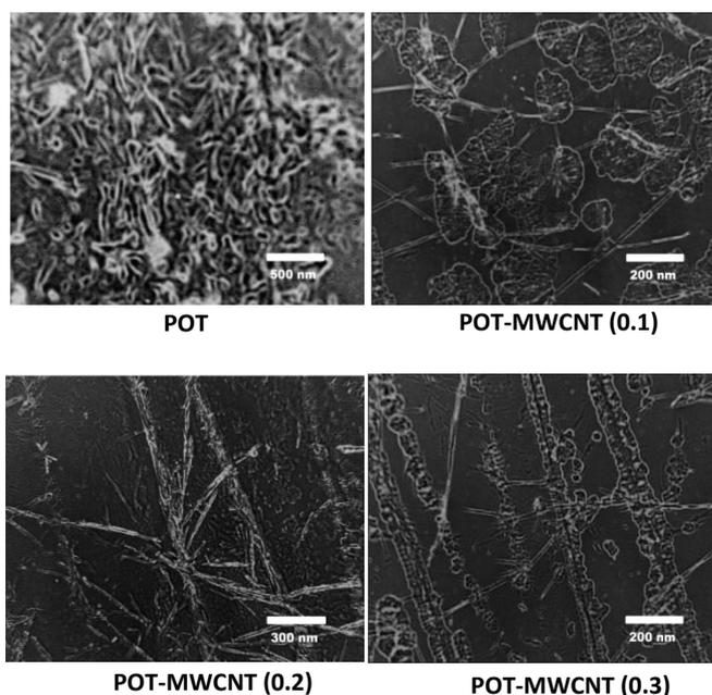
Fig. 1. SEM images of POT and POT-MWCNTs with different MWCNTs weight ratios
