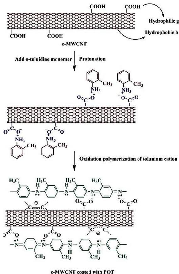
Scheme 1. In situ polymerisation of POT-MWCNT nanocomposite [9]
