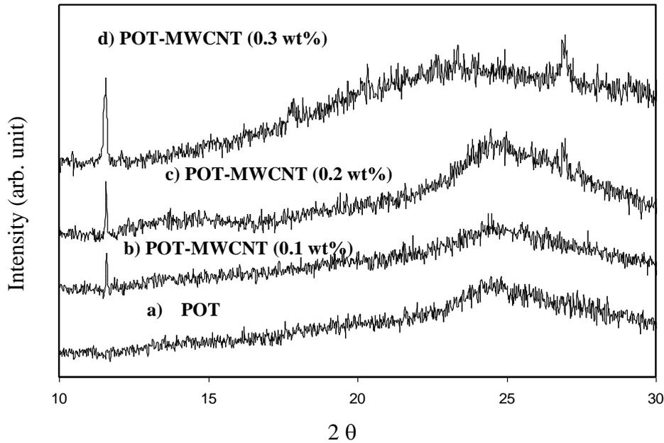
Fig. 2. XRD spectra of POT and POT-MWCNTs with different MWCNTs weight ratios
