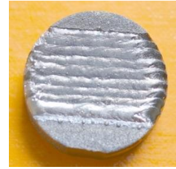
Fig. 14. Conditioned surface by successive melting strings
