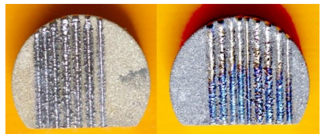
Fig. 8. Melting of the work-piece a. performed with cycle 1, b. performed with cycle 2
