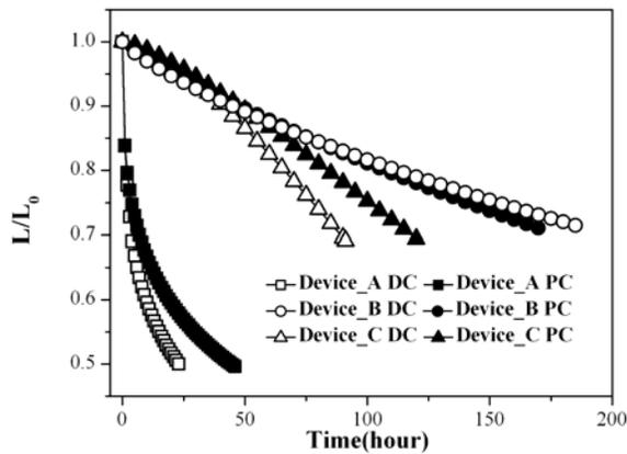
Fig. 2. Normalized luminance decay [luminance (L)/initial luminance ( $L_0$ )] of devices A-C as a function of operating time for DC and PC operation with 1:1 duty cycle, 50 Hz square wave and 5V reverse Voltage.
