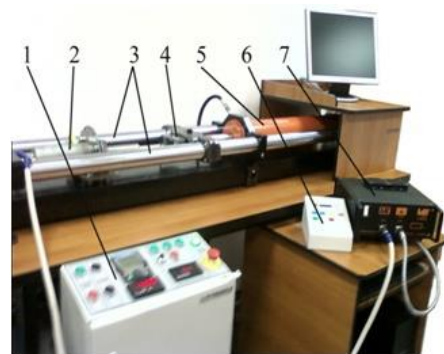
Fig. 2. Photo image of the tubes drawing bench BTL – 01.000 and of the ultrasonic equipment: 1 – control panel; 2 – oscillator system; 3 – guide columns; 4 – tube holding / drawing device; 5 – hydraulic cylinder; 6 – final level controller of the ultrasounds generator; 7 – ultrasounds generator IL 10 – 2.0 – 0.1.
