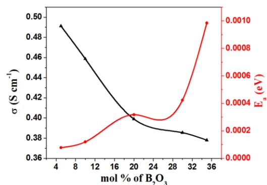
Fig. 4. Variation of  $\sigma_{dc}$  and  $E_{dc}$  with mol % of  $B_2O_3$ .
