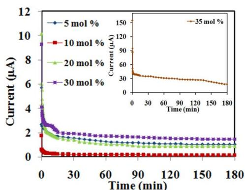
Fig. 5. Plots of DC current versus time for different mol % of  $B_2O_3$ .
