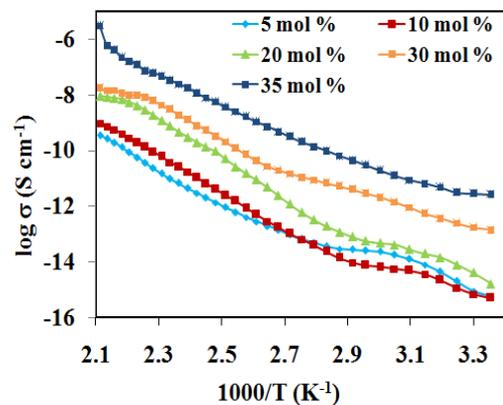
Fig. 3. Temperature dependence DC conductivity for different mol % of  $B_2O_3$ .
