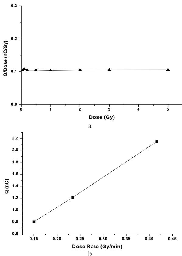
Fig. 2. Plot of a) charge over dose in C/Gy vs. the dose in Gy at -200 V with constant dose rate 0.244 Gy/min and b) charge vs. dose rate at -200 V and integrating time 30 s for  $^{60}\text{Co}$  radiation.
