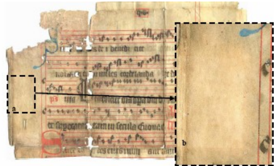
Fig. 9. Laser cleaning of area 5: a. before, b. after.
