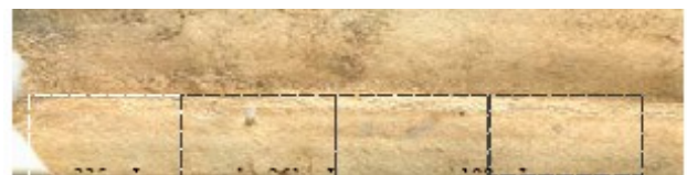
Fig. 6. Laser cleaning tests at different energies per laser spot.
