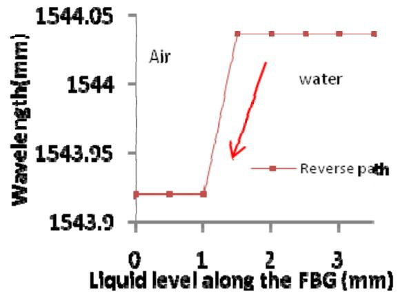
Fig.7. Wavelength response of FBG1 with liquid level falling.
