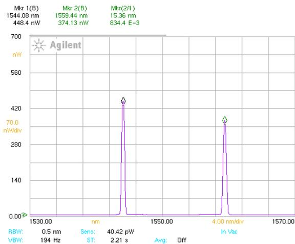
Fig. 9. Spectrum of FBG1 and FBG2 in petrol.
