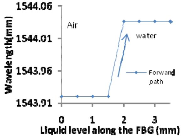
Fig.6. Wavelength response of FBG1 with liquid level rising.
