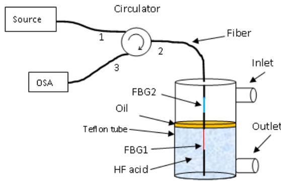
Fig. 1. Schematic of sensor packaging and etching process.
