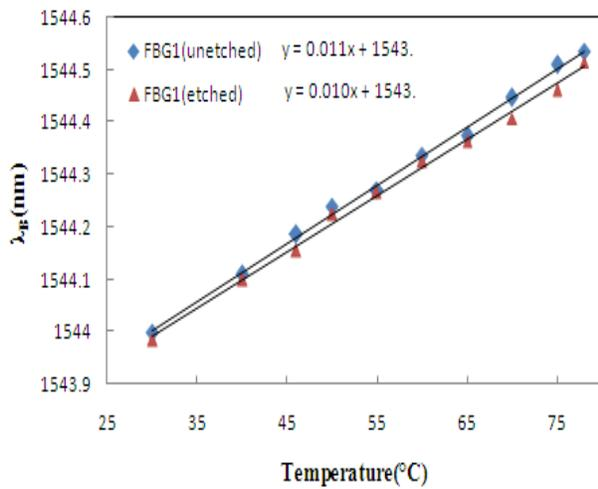
Fig. 4 .Temperature Response of FBG1.
