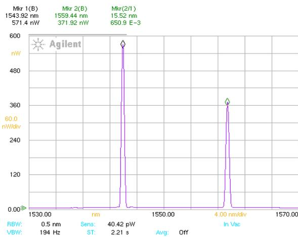
Fig. 8. Spectrum of FBG1 and FBG2 in air.
