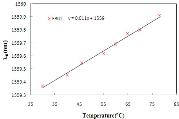
Fig. 5. Temperature response of FBG2.
