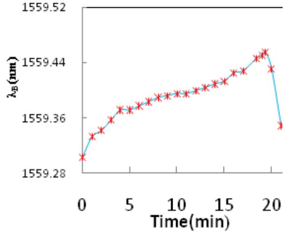
Fig. 2. Variation of  $\lambda_B$  and time during etching.
