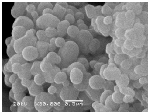
Fig. 2. SEM photograph of europium doped SMS10 phosphor.
