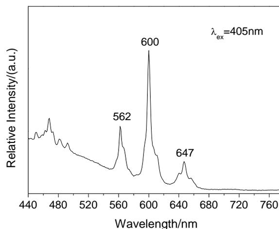
Fig. 3. The emission of the sample  $\text{LaInO}_3:0.05\text{Sm}^{3+}$  ( $\lambda_{\text{ex}}=405\text{nm}$ ).
