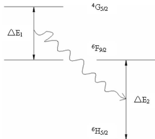
Fig. 5. Schematic diagram for the process of cross-relaxation levels of  $\text{Sm}^{3+}$  self-quenching.
