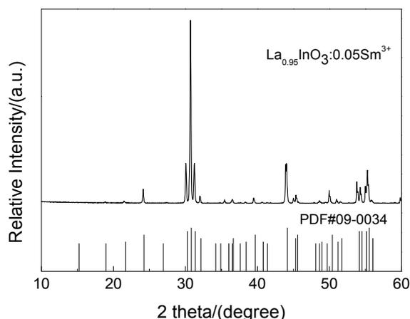
Fig. 1. XRD pattern of the sample  $\text{LaInO}_3:\text{Sm}^{3+}$ .
