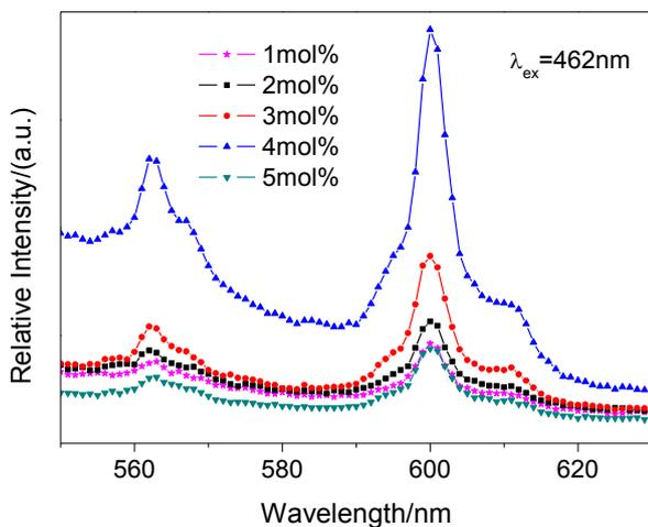
Fig. 4. The dependence of luminescence properties on  $\text{Sm}^{3+}$  concentration excited at 462nm.
