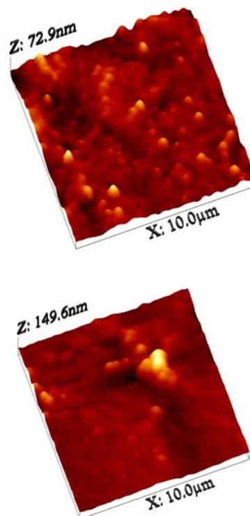
Fig. 6. AFM images of MAPLE (A) Benzil 1 film ( $R_a=5.8 \text{ nm}$ ) and (b) Benzil 3 film on silicon substrate ( $R_a=9.2 \text{ nm}$ ).
