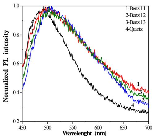
Fig. 2. PL spectra of MAPLE deposited benzil films on quartz,  $\lambda_{exc}=435$  nm.
