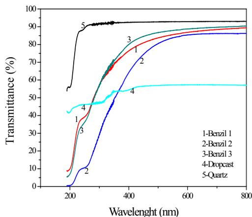
Fig. 1. UV-VIS transmission spectra of MAPLE deposited and dropcast benzil films.
