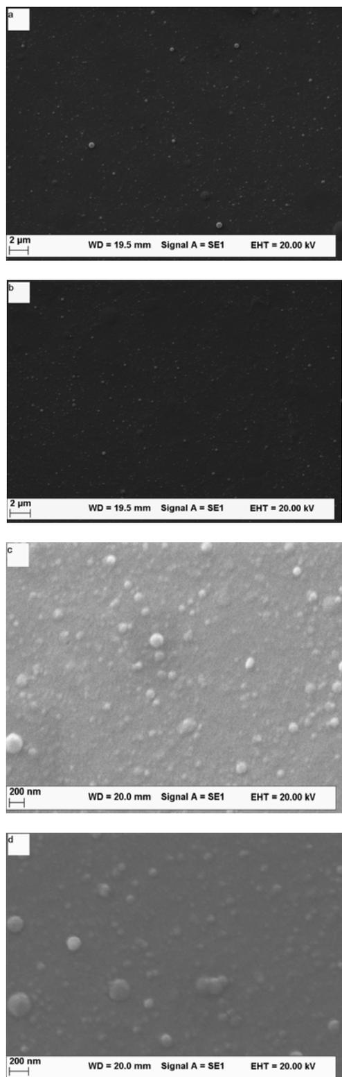
Fig. 5. SEM images of MAPLE films for two different magnitudes: Benzil 2 ((a) and (c)) and for Benzil 3 ((b) and (d)).
