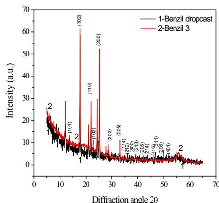
Fig. 4. XRD diagram for Benzil 3 film by comparison with Benzil dropcast layer.
