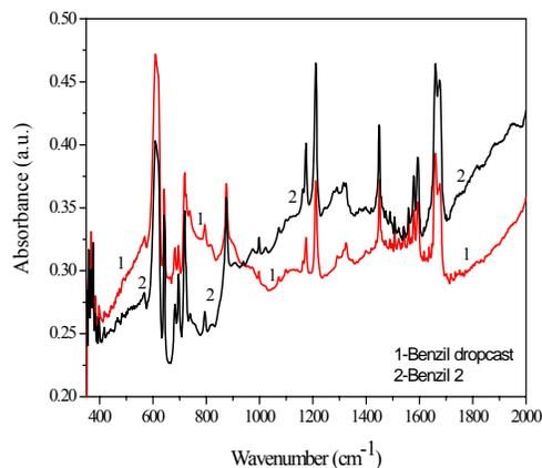
Fig. 3. FTIR spectra of Benzil 2 film by comparison with Benzil dropcast layer.
