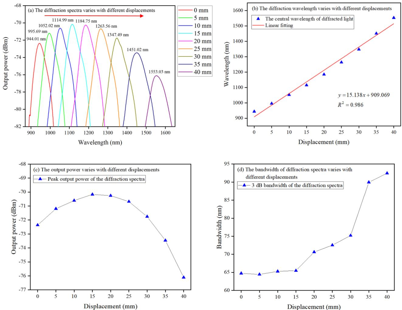
Fig. 4. Displacement experiment of the light spot toward the direction with a large period: (a) shift of the diffraction spectra, (b) variation in the central wavelength, (c) variation in the output power, and (d) variation in the bandwidth (color online)
