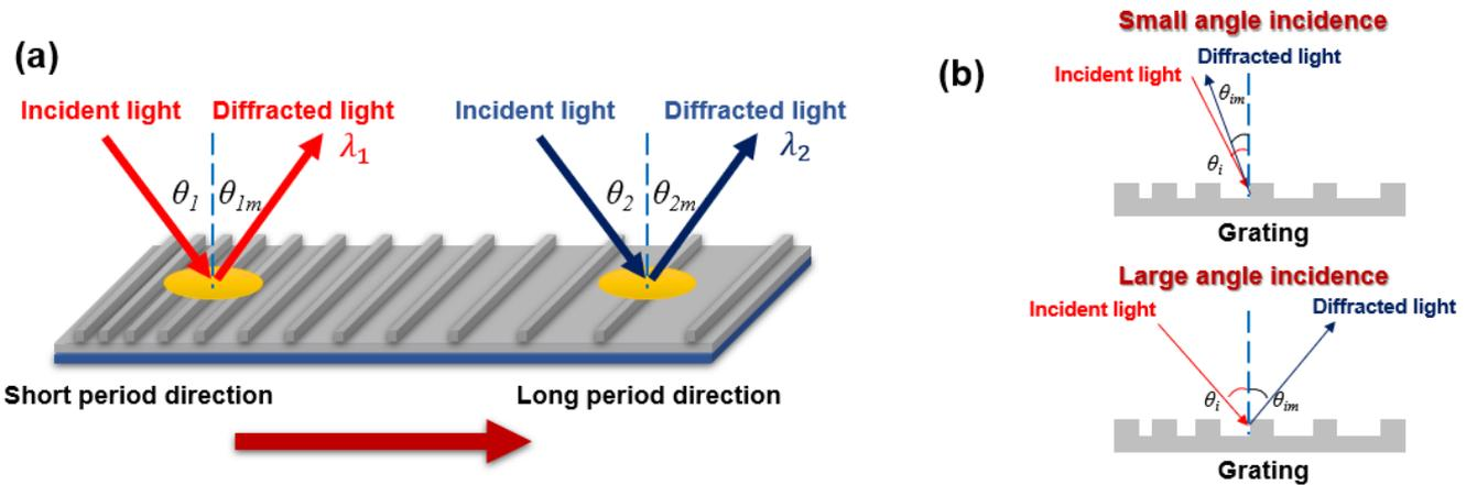
Fig. 1. Principle of proposed VSG. (a) Schematic diagram of the VSG; (b) schematic of different diffraction light angles on grating surface (color online)
