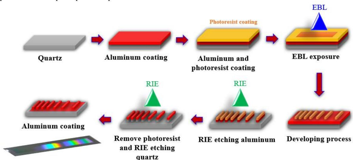
Fig. 3. Schematic of electron beam exposure manufacturing grating structure (color online)
