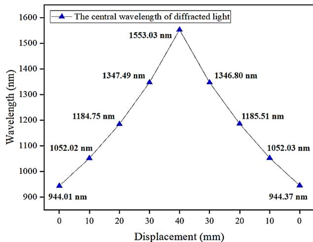
Fig. 6. Repeatability test results of displacement sensing system
