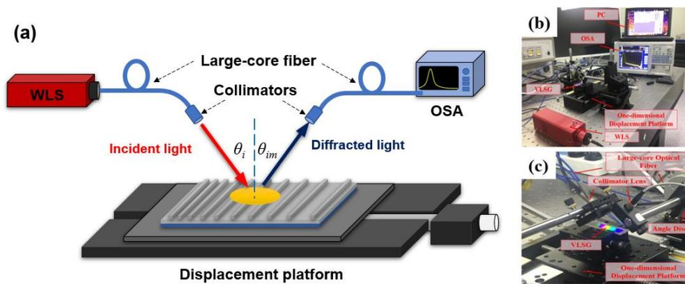
Fig. 2. The proposed displacement sensing system. (a) Schematic of displacement sensing system based on VSG; (b) overall structure of the experimental system and (c) VSG on a one-dimensional displacement platform (color online)
