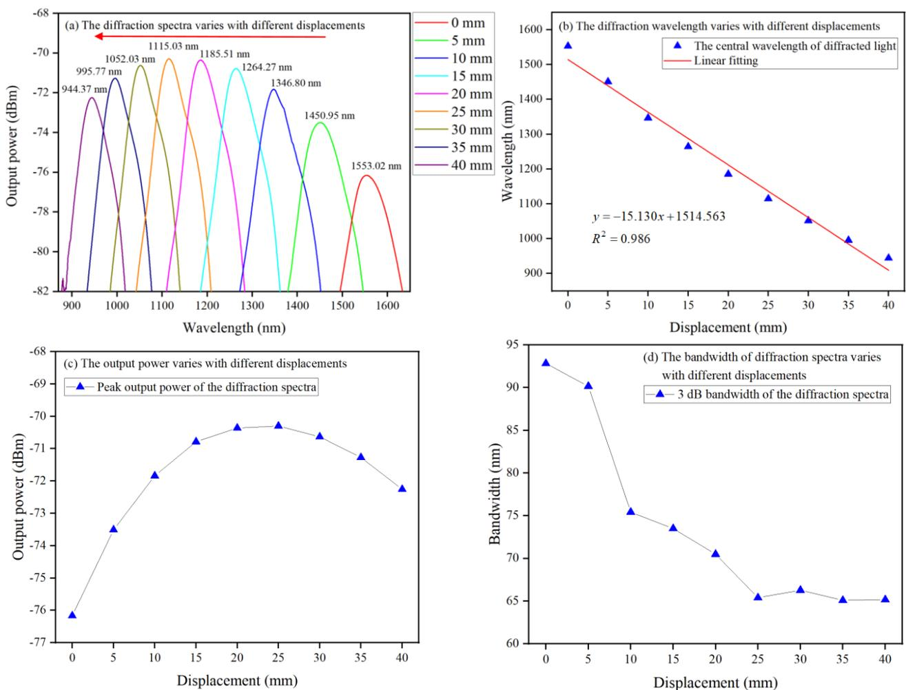
Fig. 5. Displacement experiment with the light spot moving in the direction of the small period: (a) shift of the diffraction spectra, (b) variation in the central wavelength, (c) variation in the output power, and (d) variation in the bandwidth (color online)
