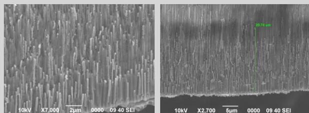
Fig. 2. SEM picture of the membrane cross section after successive gold and platinum electrochemical deposition.
