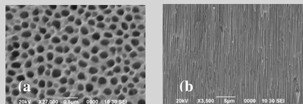
Fig. 1. SEM micrograph of Whatman nanoporous  $\text{Al}_2\text{O}_3$  membrane (a) top view; (b) section view.
