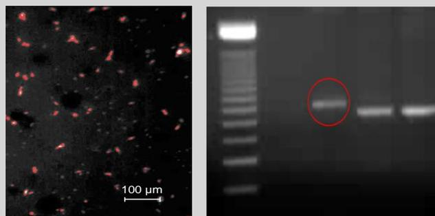
Fig. 5. (a) Nanowires detection through the fluorescence-based analysis system performed by measuring the fluorescence generated by the fluorophore-tagged PCR-amplified products immobilized on nanowires; (b) fluorescence-based gel electrophoresis migration of PCR-amplified products showing FLT3 gene mutation (inside the red circle).
