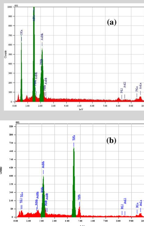
Fig. 3. EDS analysis of gold-platinum nanowires: (a) nanowires in membrane and (b) free nanowires.
